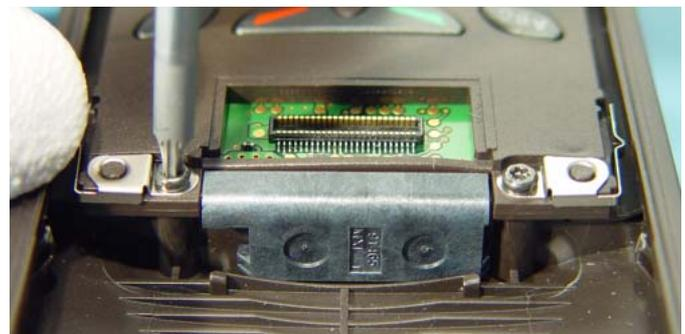
Unscrew the two screws of the Keymat Cover. When re-assembling, take care that the Battery Connector fits well.
