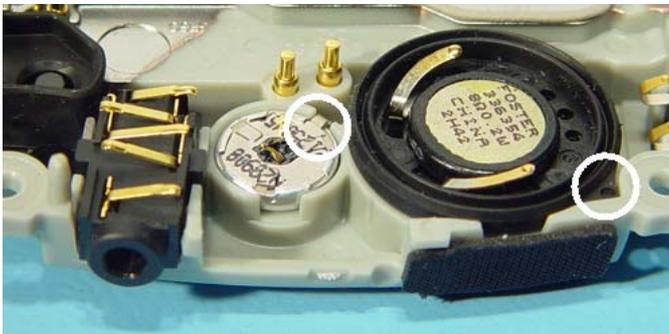
Headset Jack, Earpiece and HF-Speaker can be easily taken away. Note the guiding pins when assembling.
